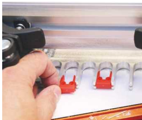
▲ The red pegs slide into the comb for setting different tail spacings
